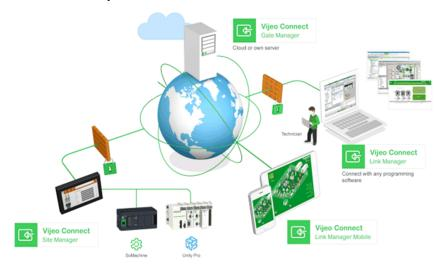
Vijeo Connect is structured to connect safely display units on the work site (SiteManager), with computers or smart devices in the office (LinkManager), over a server (GateManager).
