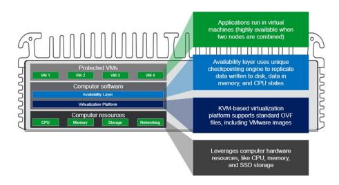
**Protected Virtual Machines:** All VMs created using ztC Edge, or those OVF or OVA formatted images imported into ztC Edge, are automatically protected by ztC Edge's availability layer:
