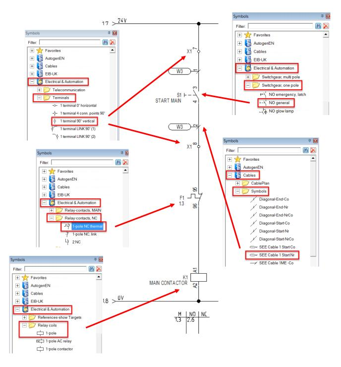
References should now appear below the relay coil (for the 3P contacts) and next to the NC thermal auxiliary contact.
