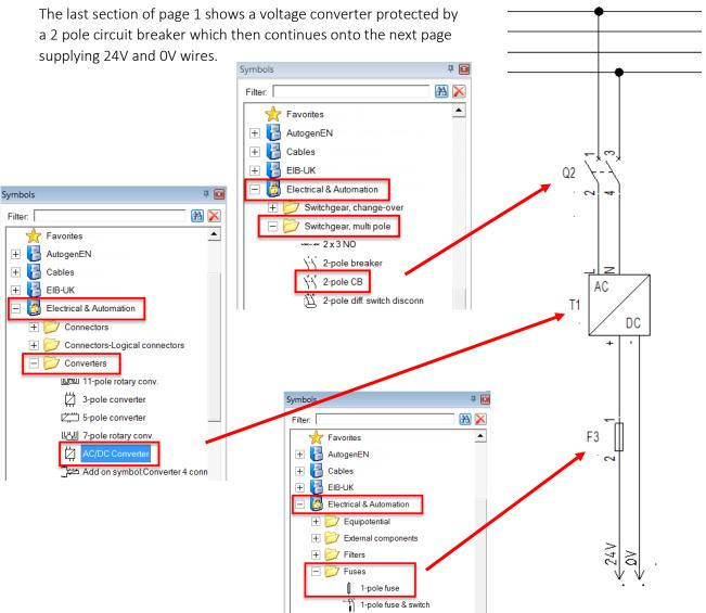
The final wires below the converter are drawn with the '1 Wire' command, double-clicking at the bottom to add the reference arrows:
