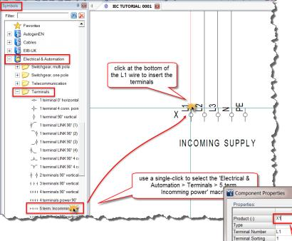
Locate the 'Symbols' panel and extend the 'Electrical & Automation' symbol database and scroll down to find the 'Terminals' folder. In here select the '5 term. Incomming power' group of terminals using a single click. Move your cursor to the end of the L1 wire and use a single-click to insert the macro.
