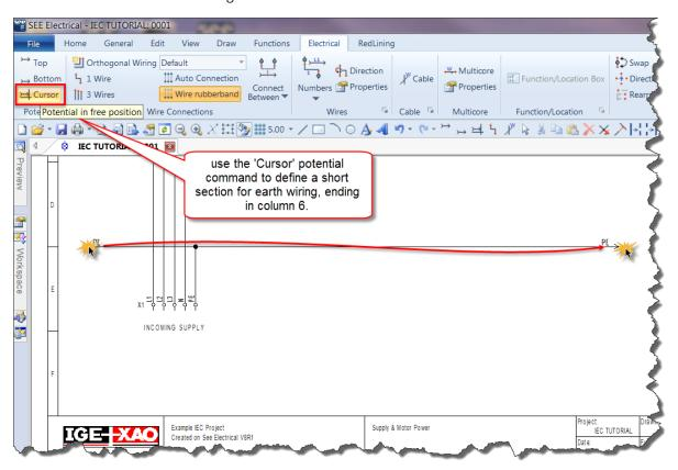
Complete this section with a '1 Wire' section from the potential to the 'PE' terminal.
