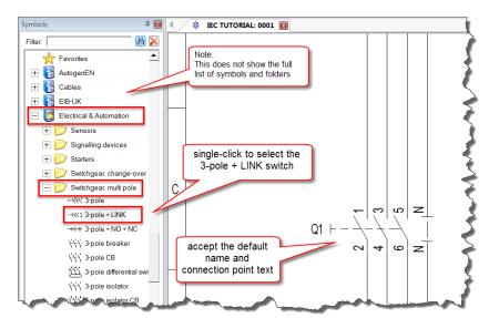
Right-click to finish inserting the symbol once it's placed on the page. Double-click on the symbol to show the 'Component Properties' dialogue to make any changes.
