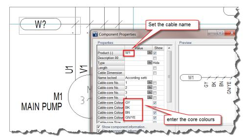
In the standard and advanced versions of See Electrical the cable core information can be stored in the type database so that the details automatically fill in when the cable type is selected.
