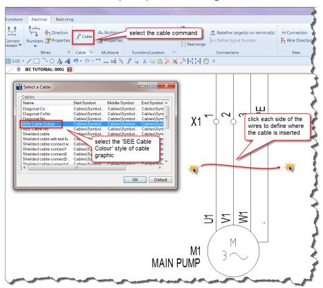
Once the position of the cables is defined the 'Component Properties' dialogue is displayed where the product name, description, type of cable, length and core details can be entered.
