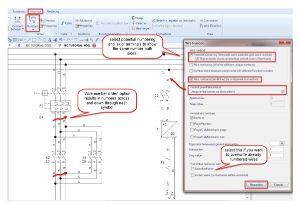
Groups of wires can still be selected after numbering to control the display of the wire number on each segment of wire.
